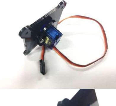
Then insert the Servo bracket holder on the top of servo holder. Now you can see Servo is secured and sandwiched between holder and bracket.
