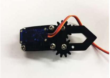
Fix the two claws on the rectangle servo bracket with two M3\*6mm screws.
