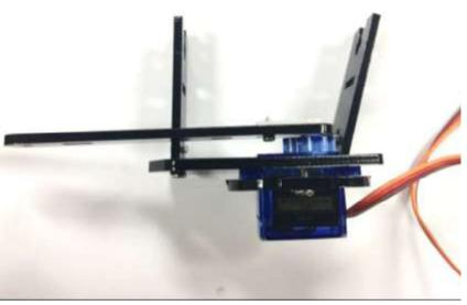
Place the two Clapboard Acrylic in the corresponding wing slot
