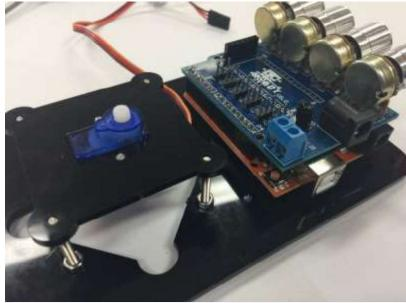
Place the Robot Arm Extension Board on the top of the Iduino UNO board.
