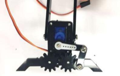
Pull the claws widely open and then insert the short arm we created in the last step and screw it firmly.
