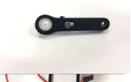
Secure the horn with tapping screw as shown on the left
