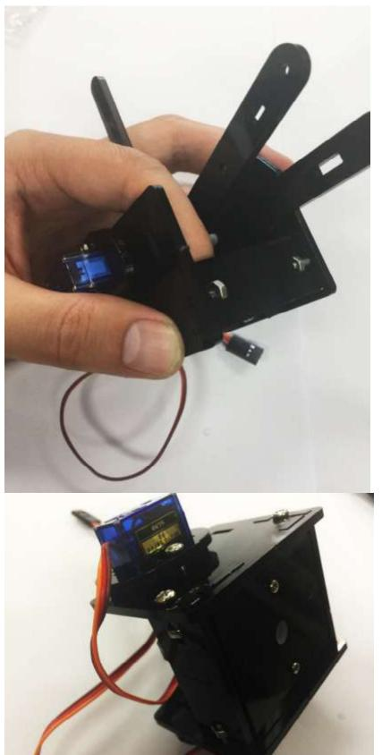
Secure the Clapboard on the Main Arm base with one pair of screw and nut.
