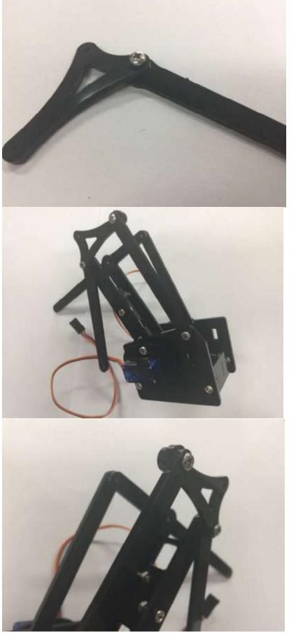
Fix the first screw as shown on the left. The circular spacer lies in the between.
