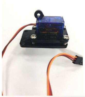
Place the rectangle bracket on the top of the Servo and secure the Servo with four M3\*8mm screws
