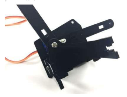
Firstly, insert the Clapboard in the corresponding slots and in the following steps it will be secured with one screw and nut on each side
