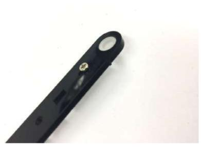
Secure the Horn on the black Main arm acrylic with M2.5 tapping screw
