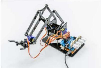
Then place the Robot Arm System on the Base servo rack and fasten it onto the base servo with a tapping screw.
