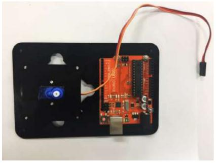
Secure the Iduino UNO Board on the Base
