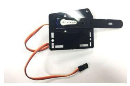
Pull out the Main Arm and put it back horizontally, this step is to ensure Servo will turn anticlockwise from this very point (0 degree) and not break the arm when power turns on to rotate
