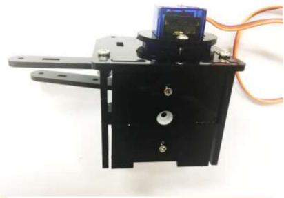
Then insert the rack base in the corresponding slot between two clapboards
