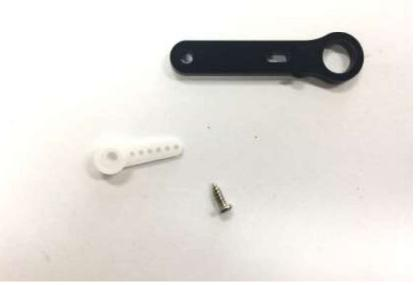
Prepare the tapping screw in the Servo package and servo horn.
