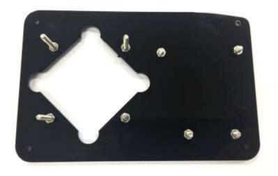
Fasten the screws and nuts as shown on the left, which are used to secure our Iduino UNO Board
