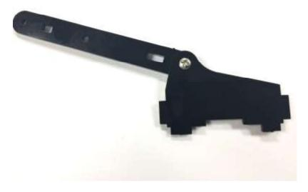
Connect two active joints by screw, remember do not over tighten the screws as they are required to rotate freely
