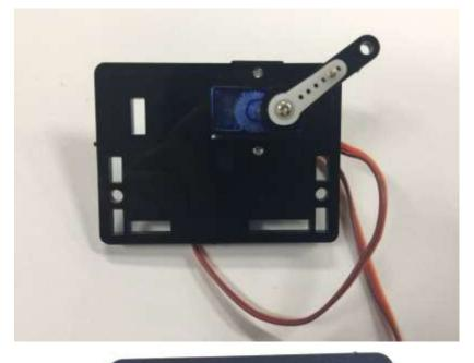
Assemble the servo on the black rack base in the same way as shown in the previous instruction.
