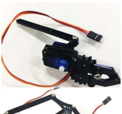
Secure the Support arm onto the Triangle connector
