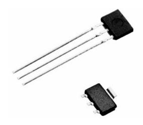
The SS49E and SS59ET Series Economical Linear Hall-effect sensors are small, versatile linear Hall-effect devices that are operated by the magnetic field from a permanent magnet or an electromagnet. The linear sourcing output voltage is set by the supply voltage and varies in proportion to the strength of the magnetic field.
