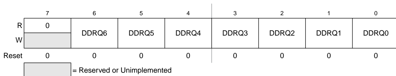
Figure 3-25. Port Q Data Direction Register (DDRQ)
