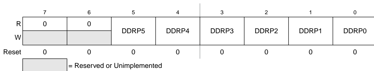
Figure 3-19. Port P Data Direction Register (DDRP)
