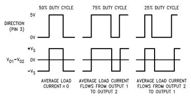
Figure 11. Locked Anti-Phase PWM Control
