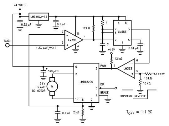
Figure 16. Fixed Off-Time Control
