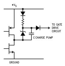
Figure 14. Internal Charge Pump Circuitry
