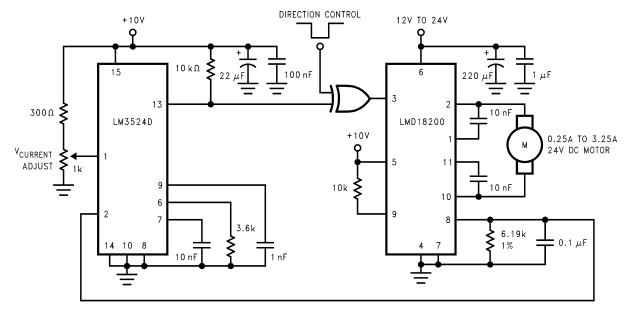
Figure 18. Locked Anti-Phase Control Regulates Torque
