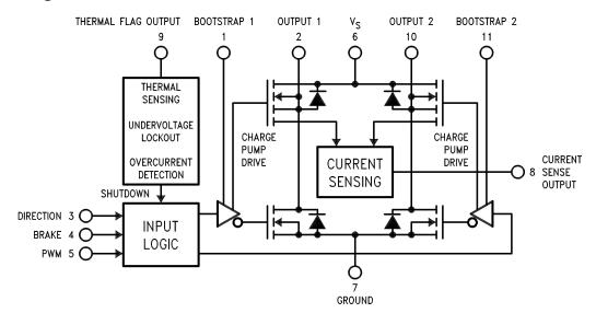
Figure 1. Functional Block Diagram of LMD18200
