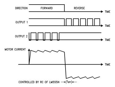
Figure 17. Switching Waveforms
