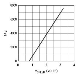
Figure 21. Motor Speed vs Control Voltage
