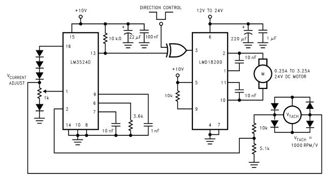
Figure 20. Regulate Velocity with Tachometer Feedback
