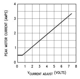
Figure 19. Peak Motor Current vs Adjustment Voltage
