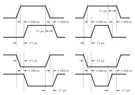
Figure 13. Transitions in Brake, Direction, or PWM Must Be Separated By At Least 1 µsec
